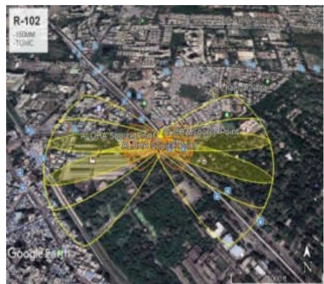
Fig. 4: Affected area, intensity of the toxic threat zone of 150 mm leak diameter in all wind direction on R-102
