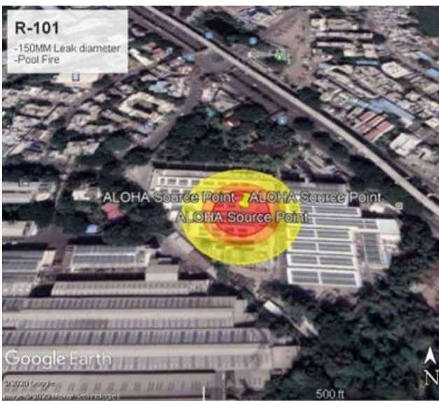
Fig. 5: Affected area, intensity of the pool fire threat zone of 150 mm leak diameter in all wind direction on R-101
