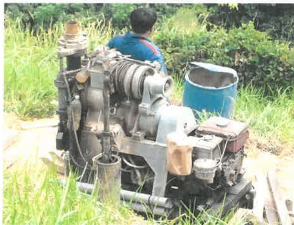
Figure 4.3.1.1 Boreholes Drilling Machine
