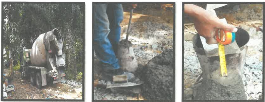
Figure 9.1 : The slump test are required at the site before the fresh concrete is fill into the framework to get the minimum strength of JKR's specification.
