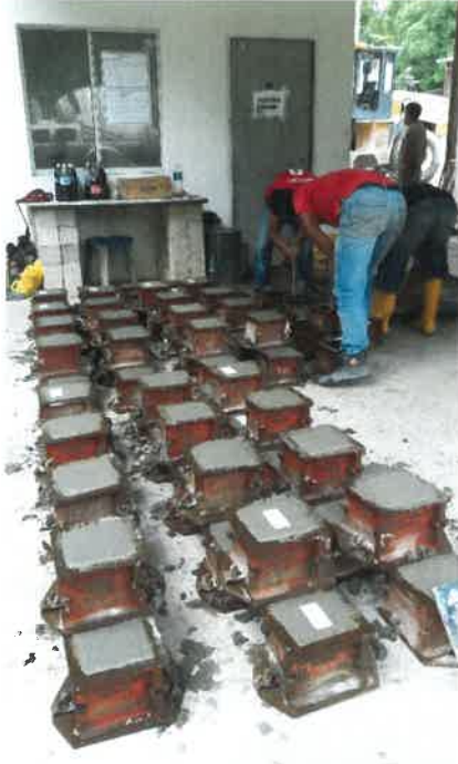
Figure 1.8 Preparing samples for cube test
