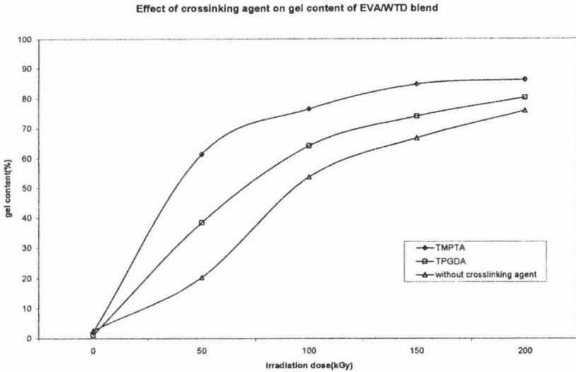
Figure 4: Effect of Crosslinking Agent on Gel Content of EVA/WTD Blend.
