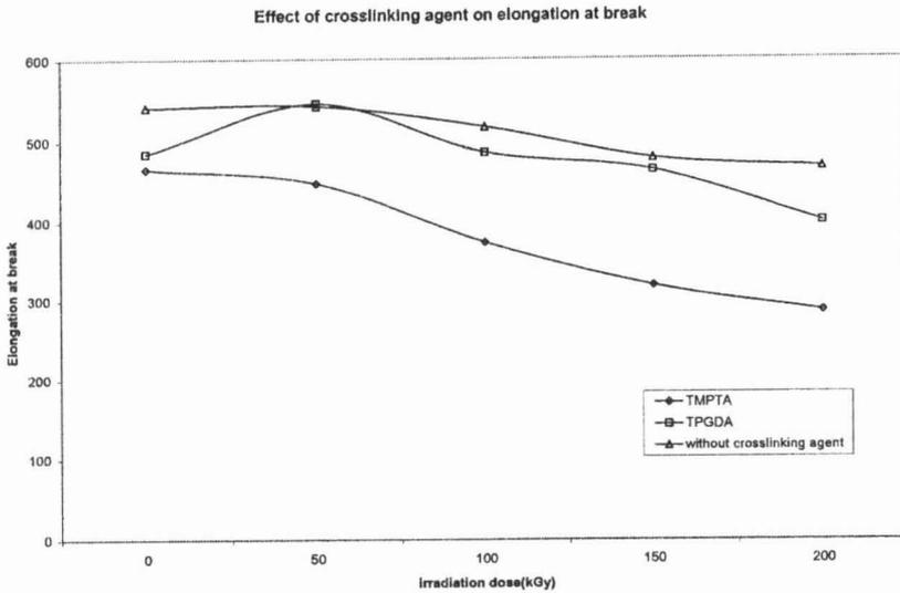
Figure 2: Effect of Crosslinking Agent on Elongation at Break of 90/10 EVA/WTD Blend.
