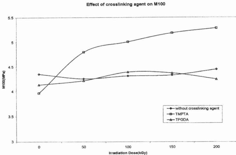
Figure 3: Effect of Irradiation on M100 of 90/10 EVA/WTD Blend.
