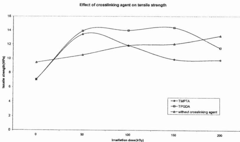
Figure 1: Effect of Crosslinking Agent on Tensile Strength of 90/10 EVA/WTD Blend.
