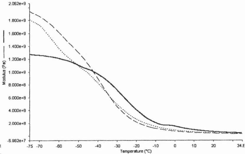
Figure 6: Temperature Dependence of Storage Modulus of 90/10 EVA/WTD Blend at 0 kGy.
