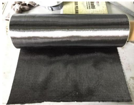
Figure 2: CFRP Sheet Roll
