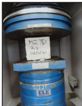
Figure 3. Compressive Strength Test Set-up
