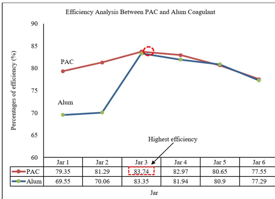
**Figure 4.** Graph of the efficiency analysis of coagulant
