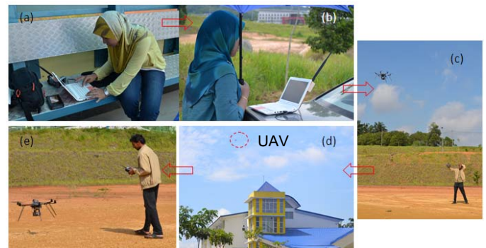
Figure 10: Procedure of data acquisition sequence using rotary wing UAV (a) Planning waypoint, (b) Planned data linked to the UAV, (c) Take off autonomously and (d) Aerial photography (e) Landing Autonomously
