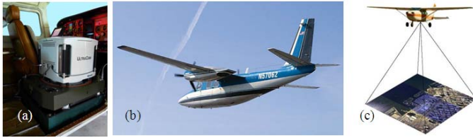
Figure 2: (a) Aerial camera system mounted in an aircraft, (b) Aircraft used for aerial photography, (c) Aerial photography. Source: [17].
