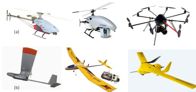
Figure 3: Example of different types of civilian unmanned aerial vehicle (UAV) (a) Rotary (b) Fixed-wing
