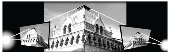
Figure 1: Two successive photographs (left and right photograph) for 3D measurement and modeling. Source: [22]
