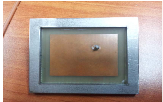
Figure 4. The fabricated microstrip antenna with PEC cavity applied.
