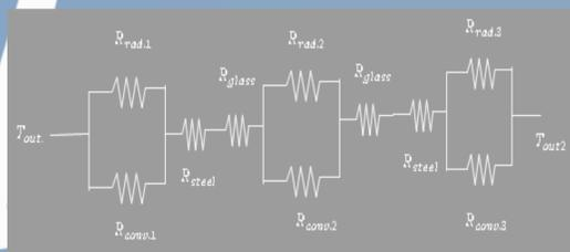
$$\dot{Q}_{cond} = -kA \frac{\Delta T}{\Delta x} \quad \text{----- equation (1)}$$
