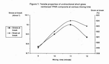
The stress and strain increased with mixing time and reached the maximum values of about 10 MPa after 11 minutes respectively and decreased thereafter. These observations indicate that the glass fibres required certain duration of time to disperse into the matrix.
