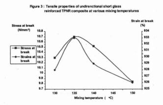
From this figure, it can be seen clearly that when the temperatures are higher than the optimum mixing temperature the tensile stress and strain of the composite decreased as a result of phase separation<sup>6</sup>.
