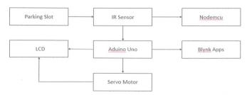
Figure 1: Block Diagram of Iot Based Parking System Using Esp8266
