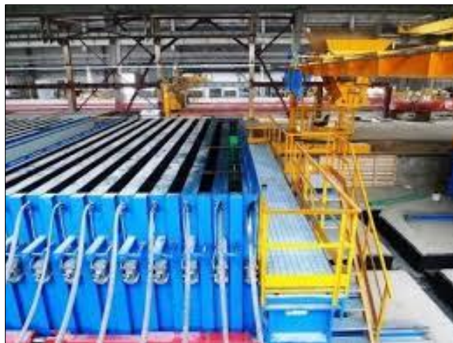
Figure 3.5 : Example Of Mould Precast Concrete
