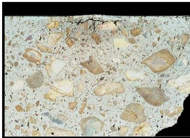
Figure 2.16: the slab surface contain blister
