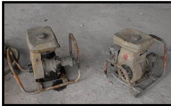
Photos 3.20 : This concrete vibrator is used during the concreting work is carried out.
