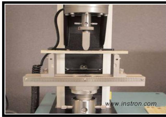
Photos 2.5 : Example of bend testing under a three-point bend arrangement.
