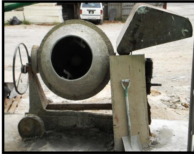
Photos 3.23 : This concrete mixer machine is used to batching concrete manually.
