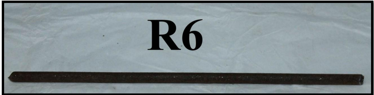
Photos 3.41 : Mild Steel Reinforcement Bar 6 Ø
