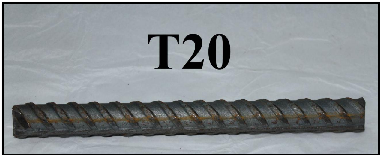
Photos 3.46 : High Tensile Steel Reinforcement Bar 20 Ø
