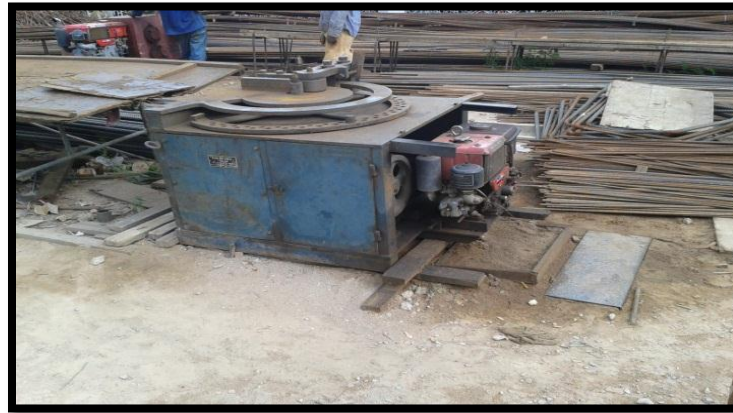
Photos 3.14 : Bar Bending Machine used at construction site Felda, Bangi.
