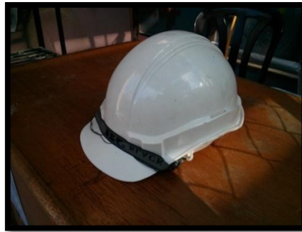
Photos 3.6 : Safety helmet to protect head from falling objects
