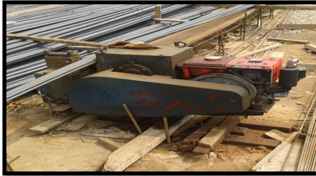
Photos 3.15 : Bar Cutter Machine used at construction site Felda, Bangi.
