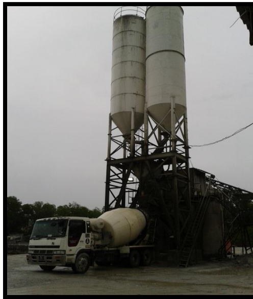
Photos 2.14 : Concrete Batching Plant from PA Concrete Sdn Bhd used in Project Hotel & Apartment Felda, bangi, Selangor.
