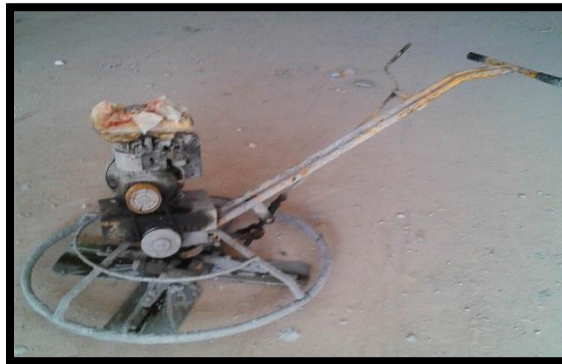
Photos 3.22 : One of power trowel machine used for floor hardener work.
