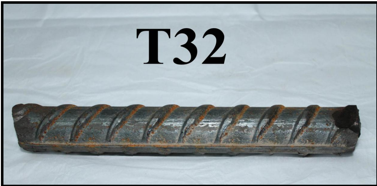
Photos 3.48 : High Tensile Steel Reinforcement Bar 32 Ø
