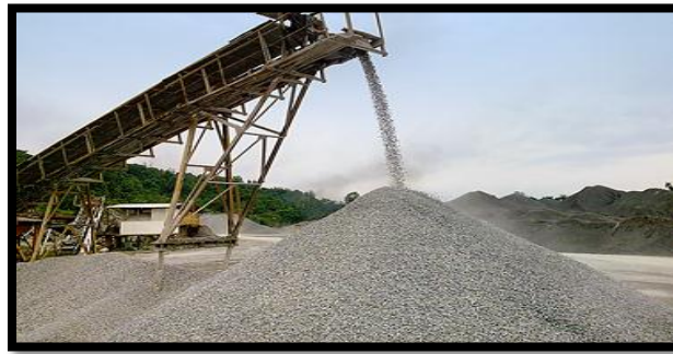
Photos 2.11 : Crushing process to be coarse aggregates
