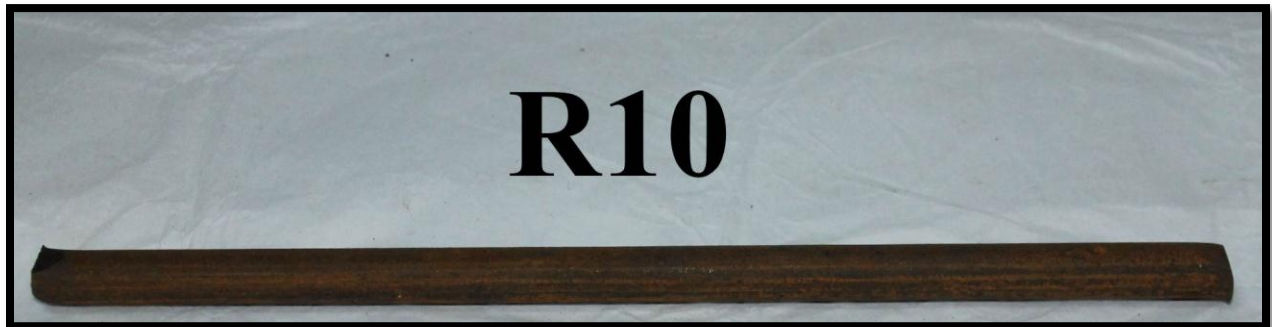
Photos 3.42 : Mild Steel Reinforcement Bar 10 Ø
