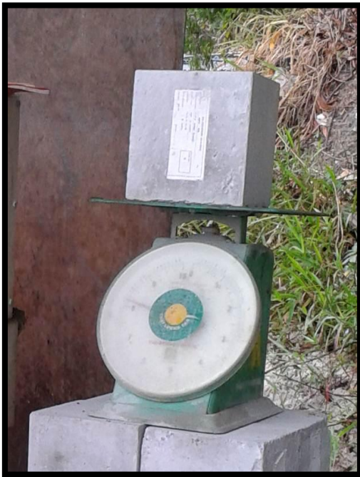
Photos 3.94 : Weight scales for concrete cubes.
