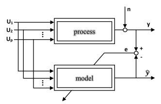
Fig. 2. System Identification block diagram.
