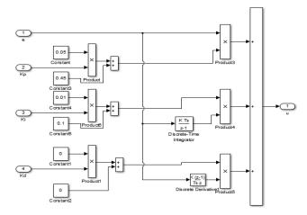
Fig. 8.PID controller block model components under fuzzy PID block.
