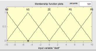
Fig. 11. Input membership function for error rate in temperature.
