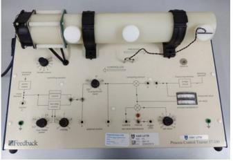
Fig. 1.PT326 process trainer heating system.
