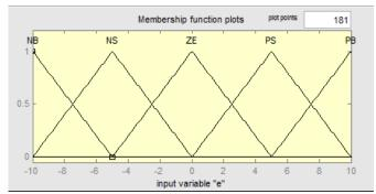
Fig. 10. Input membership function for error in temperature.
