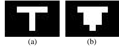
Figure 1. The comparison between area and convex area calculation image of sample object. Image (a) shows the calculation for area and (b) shows the calculation for convex area.
