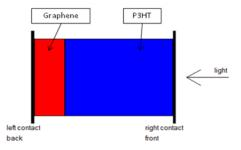
Fig. 1. Solar cell structure of P3HT/Graphene layer
