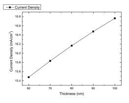
Fig. 5. The short circuit current density  $(J_{sc})$  for every thickness
