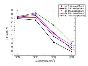
Fig. 6. Fill Factor (FF) for every thickness and concentration of P3HT
