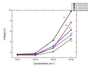
Fig. 4. The open circuit voltage  $(V_{\alpha})$  for every thickness and concentration
