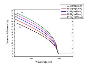
Fig. 3. The quantum efficiency (QE) at different thickness of the active layer.
