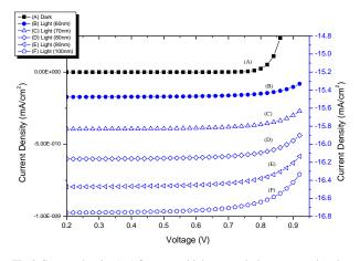
Fig 2 Current density  $(J_{sc})$  for every thickness at dark current and under illumination at a hole concentration of  $1.0 \times 10^{16} \text{ cm}^{-3}$ .
