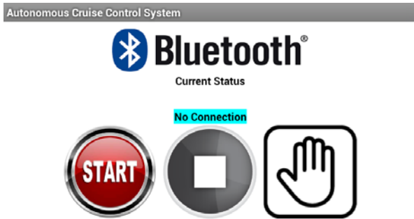
Fig. 9. Driver interface for Autonomous Cruise Control System
