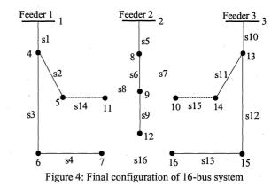
The stage II procedure involve branch exchange operations. The branch exchanged method are to compute the change of power losses by operating a pair of switches (close one and open another one at the same time). The pair of the switch are between s7 and s15, s8 and s14, s16 and s4.
