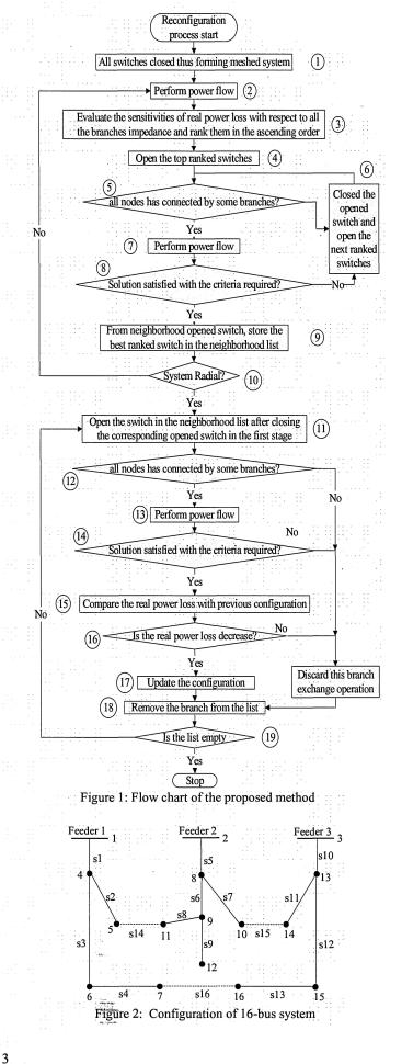
The sensitivities values of remaining candidate switches are shown in Table III. From Table III, it can be seen that, the top ranked switch is s8. Branch s14 are stored in the neighborhood switch list. Power flow was performed. At this iteration the system configuration in radial network. Procedure of the Stage I are completed. The opened switches at end of Stage I are s16, s7 and s8.
