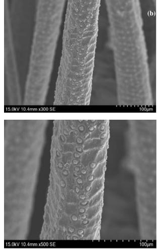
Fig. 2: SEM micrograph of Areca nut husk (a) with magnification of  $300 \times$  and (b)  $1000 \times$
