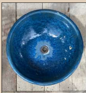
Figure 3: The top view of vessel sinks fired at 1180°C of gloss temperature
