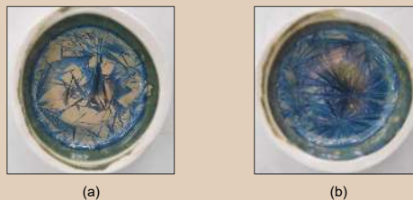
Figure 2: The sample of (a) 17% conventional silica and (b) 17% of RSA with gloss temperature at 1180°C and 1060°C of crystallization temperature with 5 hours of soaking period.
