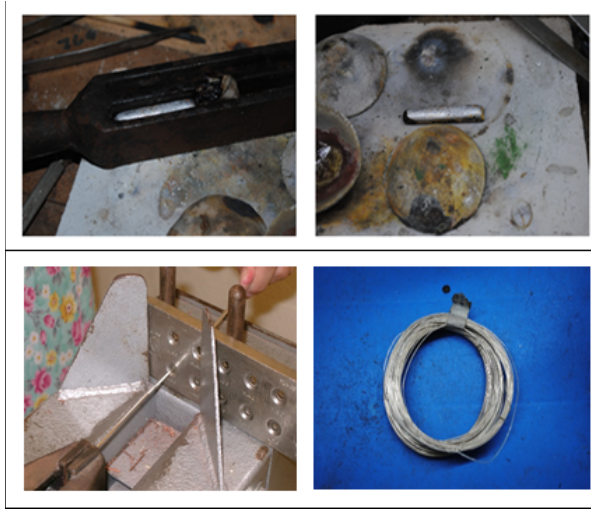
Figure 59: Silver bar inside a groove will be pulled to make a small wire Drawing the plate is a machine to make a wire to get a suitable size for weaving purposes. The requirement size for weaving is 0.5mm.
