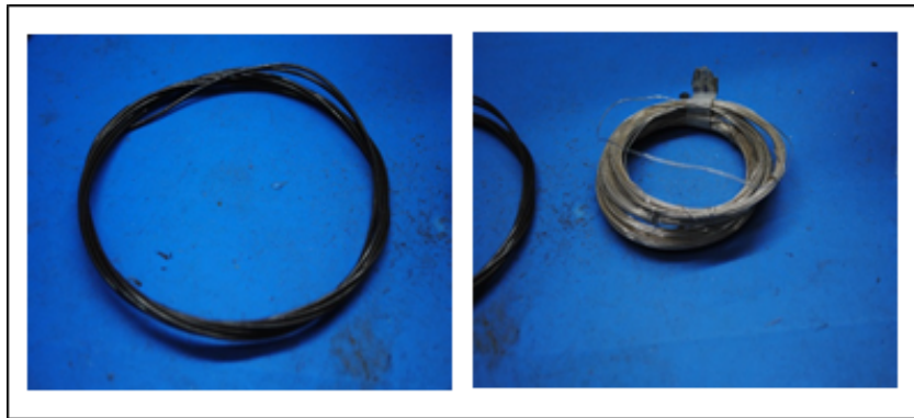
Figure 56: Two different sizes of wire are ready to weave. The size of warp is 1.5mm and the size of weft is 0.5mm, one vertical (the warp) and one horizontal (the weft).
