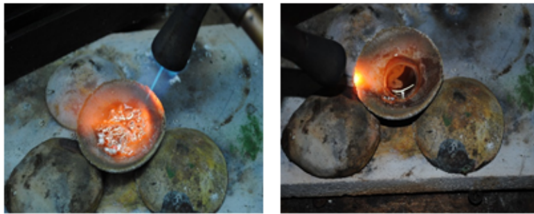
Figure 59: Silver melts with acetylene gas to get a small rod or bar
