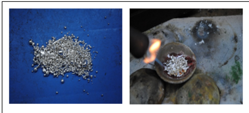
Figure 58: Silver is the main material to make a jewelry product because it's cheap and easy to get. Silver will alloy with copper to get sterling silver to make a wire.
