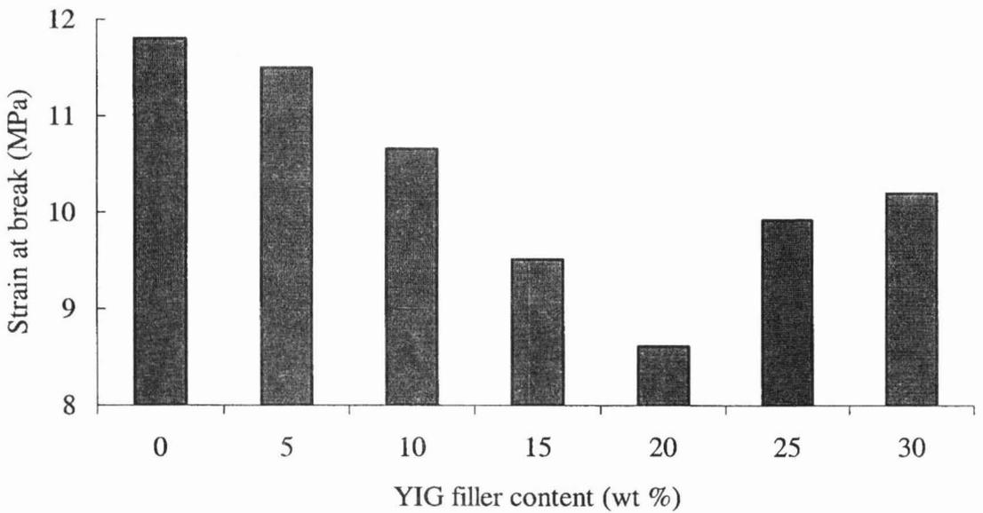
**Figure 3** The variation of strain at break for all composites as a function of filler content
