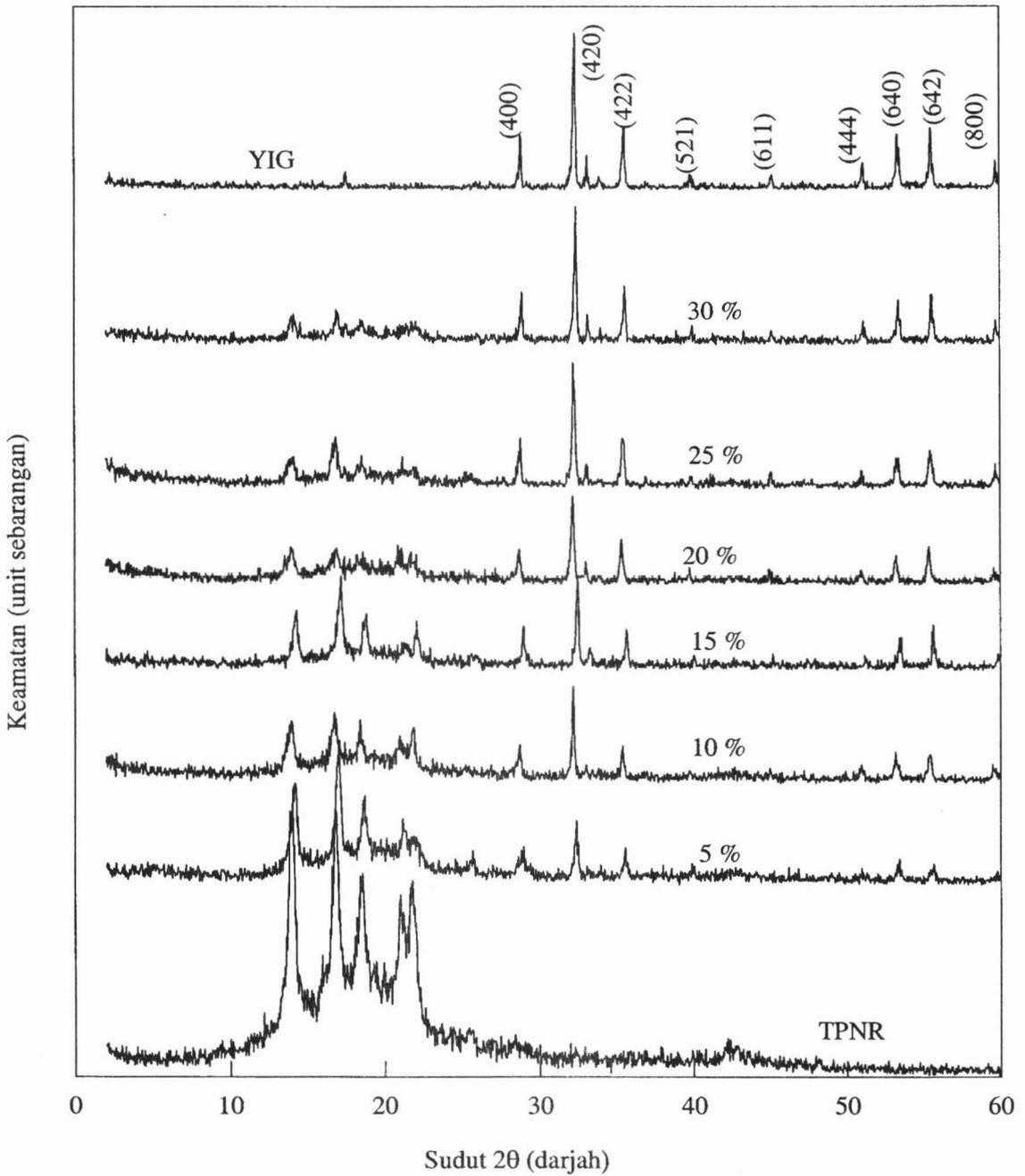
**Figure 1** X-ray diffractogram at room temperature for the pure YIG ferrite, PP/NR matrix and the composite of PP70NR30 that contain 5 to 30 weight percent of YIG ferrite filler.
