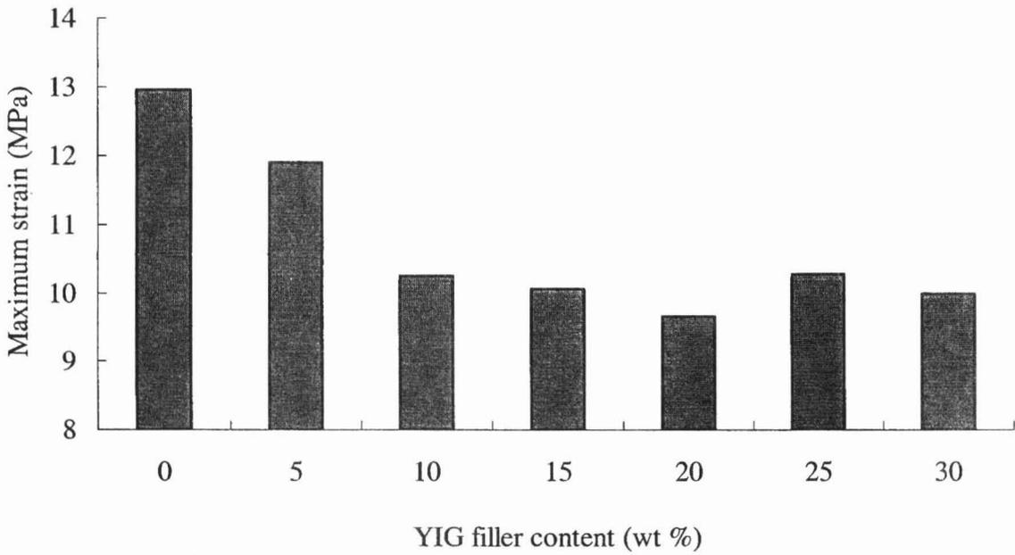
**Figure 2** The variation of maximum strain for all composites as a function of filler content
