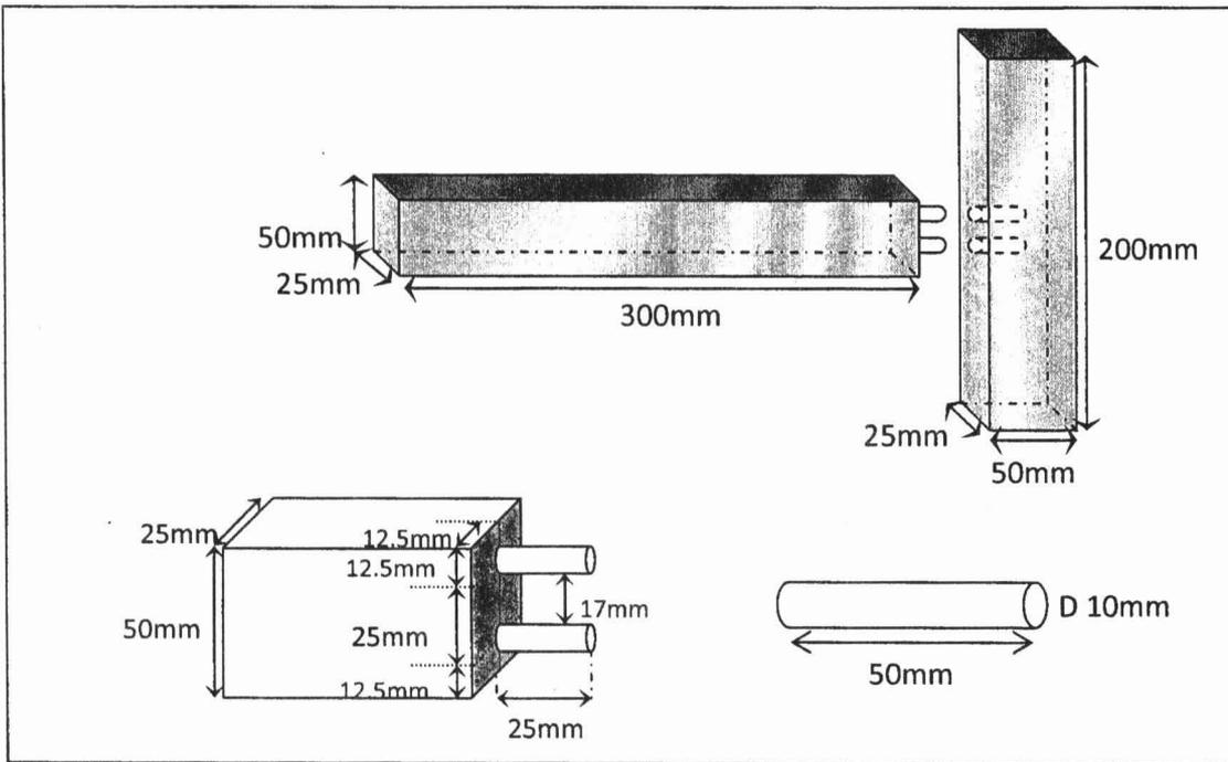
Figure 1: The dimensional of dowel joint
