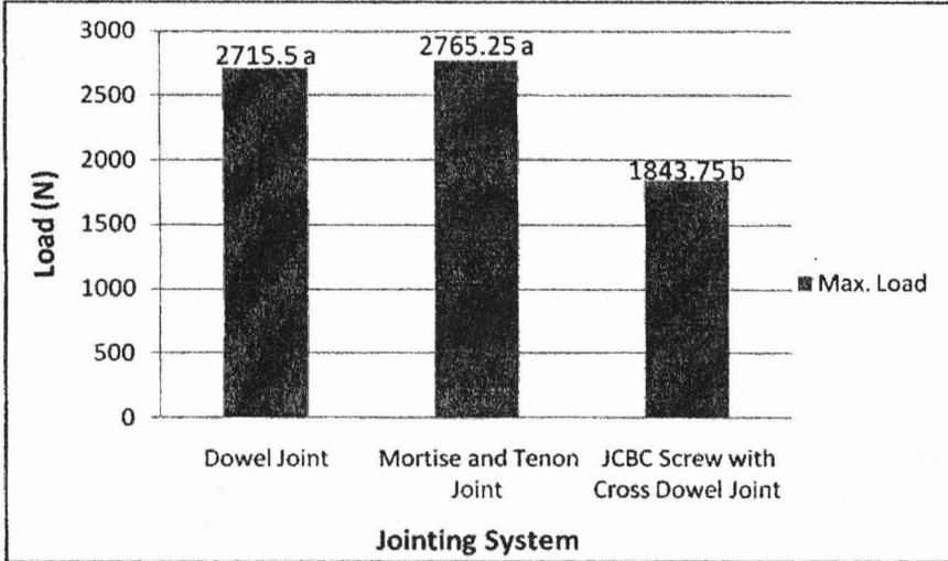
Figure 5: Comparison Between The Jointing System For Tensile Test
