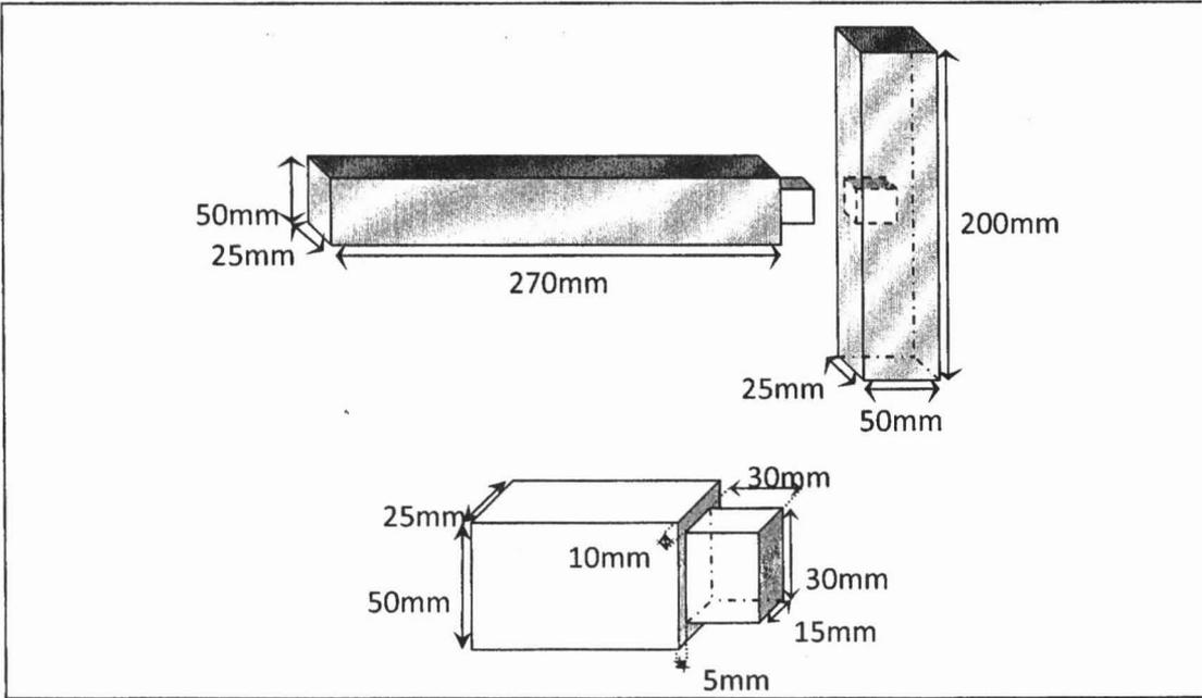
Figure 2: The dimensional of mortise and tenon joint
