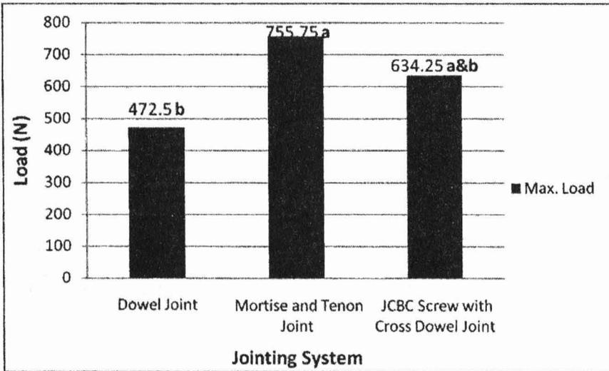
Figure 6: Comparison Between The Jointing System For Compression Test
