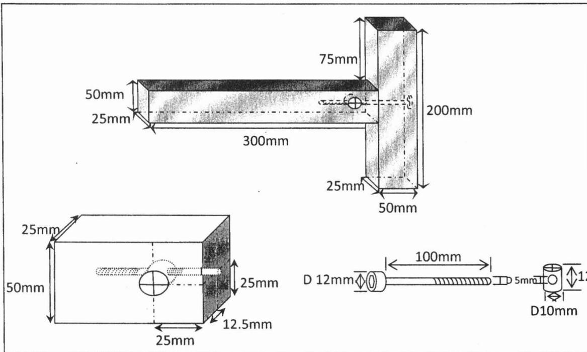
Figure 3: The dimensional of JCBC screw with cross dowel joint
