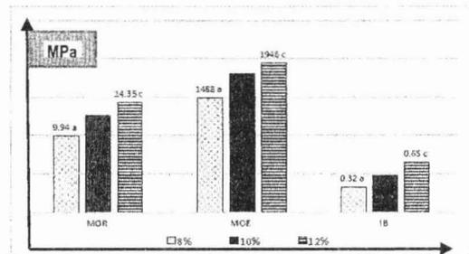
Figure 1: Effect of resin content on mechanical properties
