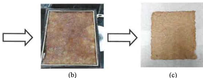
Fig. 2. (a) Preparation of materials; (b) Preparation of banana paper; (c) Banana fibre paper.
