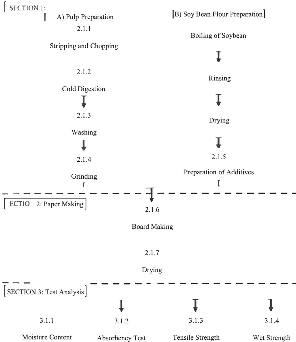
Fig.1 Flowchart of the process for paper making
