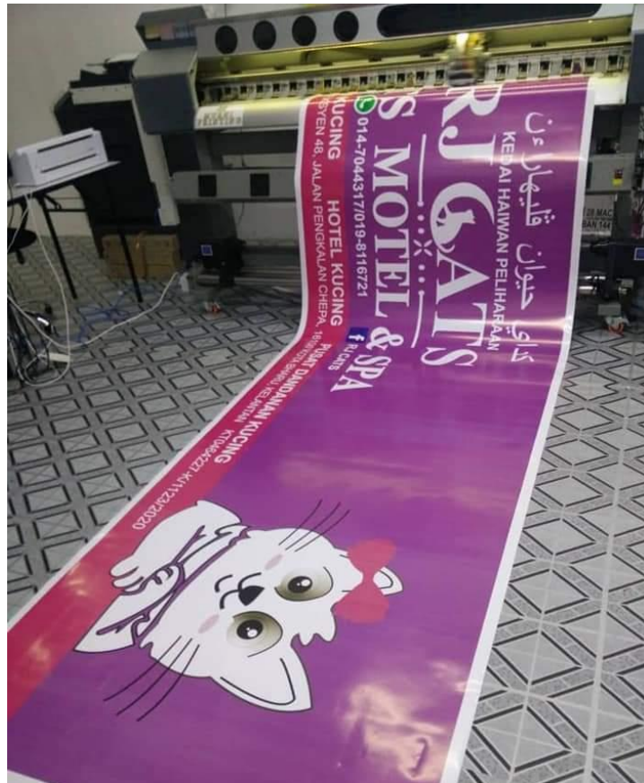
Figure 15: The process to print the banner by using machine at Murni Printing Enterprise.
