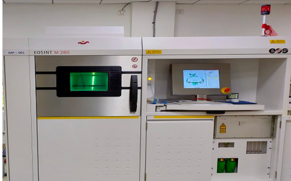
Figure 2: EOSINT M280 DMLS Machine used for manufacturing.
