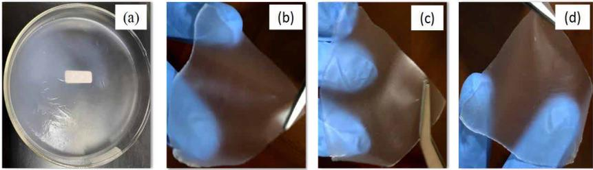
**Figure 3: The Selected Pictures of SPE Films (a) Pure Corn Starch, (b) 5 wt. % of  $\text{NaHSO}_3$ , (c) 15 wt. % of  $\text{NaHSO}_3$  and (d) 25 wt. % of  $\text{NaHSO}_3$  (Source by Author)**
