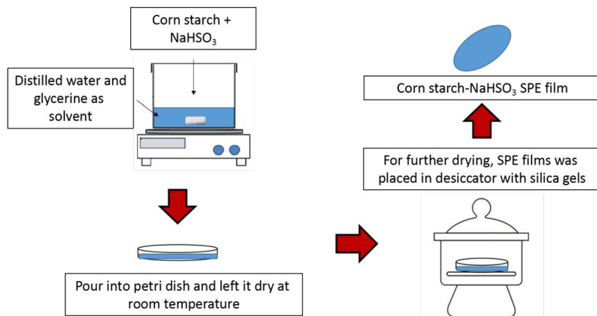
**Figure 1: The Overall Process for SPE Preparation**
