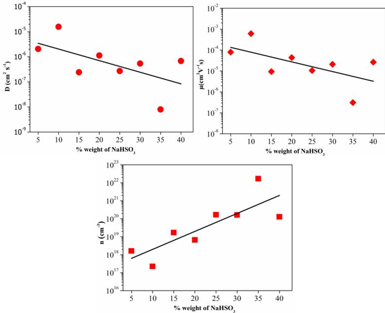
**Figure 7: The Trend of Diffusion Coefficient, D, Mobility of Ion Charges, μ and Number Density of Charge Carriers, n Against NaHSO<sub>3</sub> Concentration**
