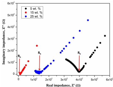
**Figure 4: The Images of Bulk Resistance,  $R_b$  SPE Films Containing Different Amounts of  $\text{NaHSO}_3$  (wt. %)**
