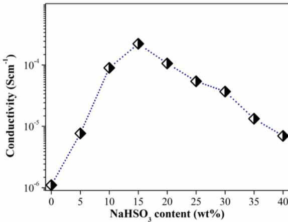
**Figure 5: Effect of NaHSO<sub>3</sub> Content on the Conductivity of Electrolyte at Room Temperature**
