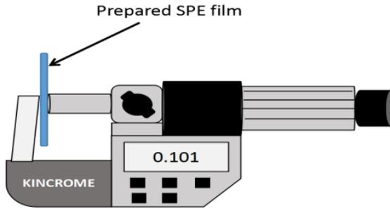
**Figure 2: The Thickness of SPE Films are Measured**
