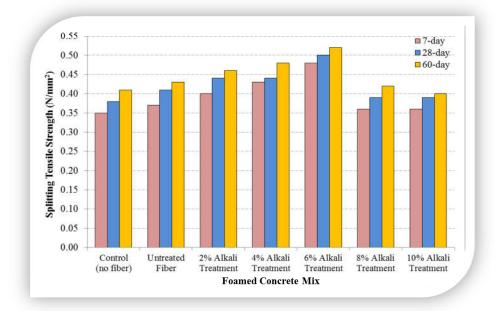
Figure 8: Influence of alkali treatment of coir fiber on splitting tensile strength for 1100kg/m<sup>3</sup> density
