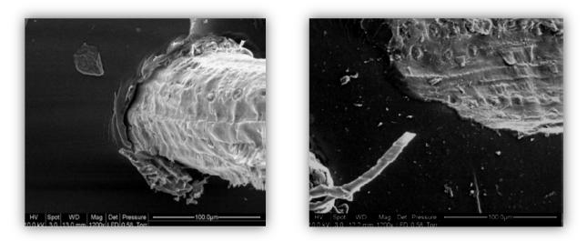
Figure 10: SEM results of coir fiber-cement interface: untreated (left) & treated (right)
