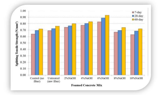
Figure 9: Influence of alkali treatment of coir fiber on splitting tensile strength for 1400kg/m<sup>3</sup> density
