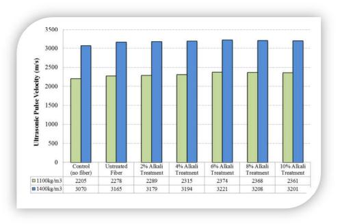
Figure 5: Influence of alkali treatment of coir fiber on ultrasonic pulse velocity of foamed concrete
