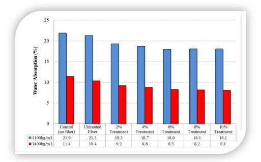
Figure 3: Influence of alkali treatment of coir fiber on moisture absorption capacity of foamed concrete
