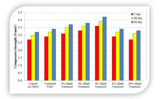
Figure 6: Influence of alkali treatment of coir fiber on compressive strength for 1100kg/m<sup>3</sup> density
