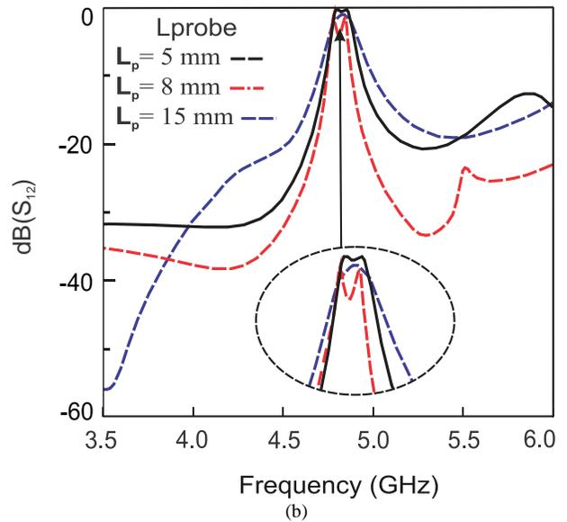
Fig 6: Effect of varying length of the probe, (a)  $S_{11}$  parameters and (b)  $S_{12}$  parameters.
