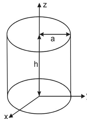
Fig 1: Geometry for circular cavity
