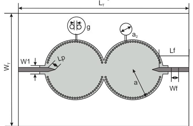
Fig 3: Geometry of the proposed filter, top view.
