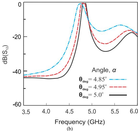
Fig 5: Effect of varying angle,  $\alpha$  (deg), (a)  $S_{11}$  parameters and (b)  $S_{12}$  parameters.
