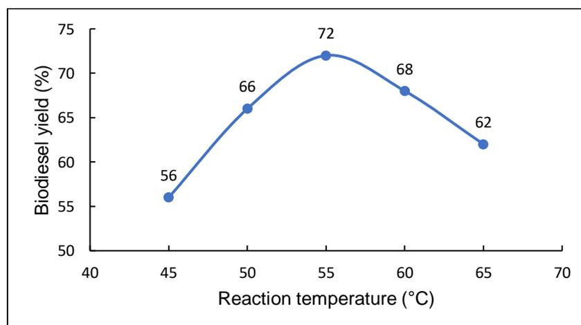
Figure 3. Biodiesel yield at different temperatures.
