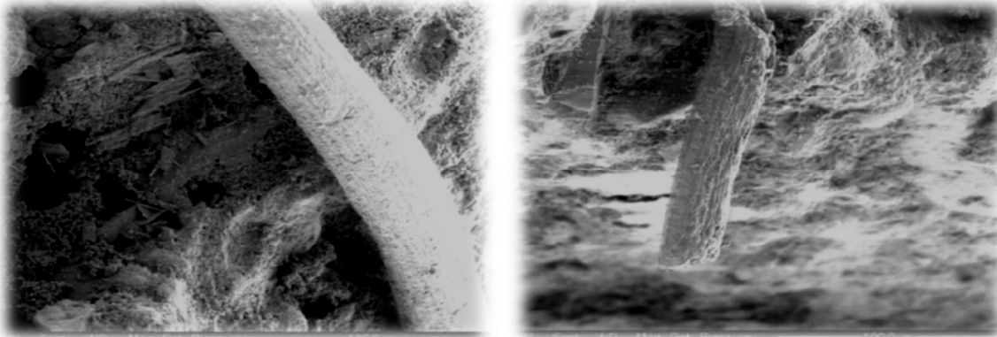
Figure 17: Retreat of empty fruit bunch fiber from the cement matrix
