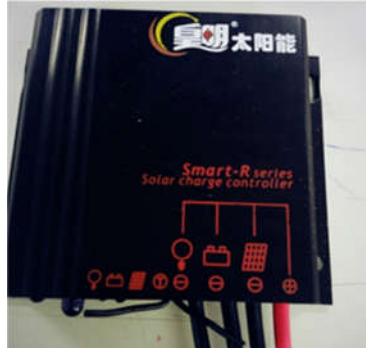
Figure 6: Controller of Himin Solar Company China (Himin Solar Co., Ltd, 2017)
