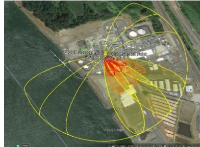
Figure 13: Area affected at 500 bar from 25 mm leakage.
