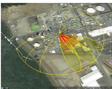
Figure 8: Area affected at 500 bar from 10 mm leakage.
