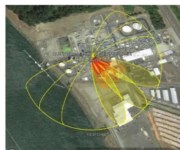
Figure 9: Area affected at 100 bar from 25 mm leakage.
