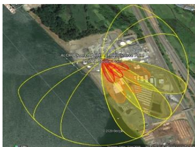
Figure 15: Area affected at 200 bar from 160 mm leakage.
