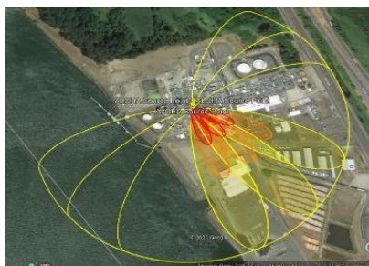
Figure 14: Area affected at 100 bar from 160 mm leakage.
