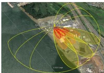
Figure 16: Area affected at 300 bar from 160 mm leakage.
