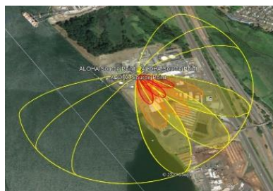
Figure 17: Area affected at 400 bar from 160 mm leakage.
