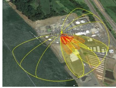
Figure 11: Area affected at 300 bar from 25 mm leakage.
