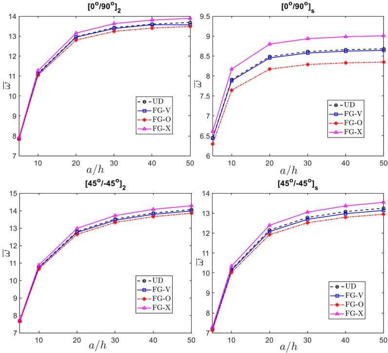
Figure 4: The variation of the non-dimensional fundamental frequency of cross-ply and angle-ply laminated FG-CNTRC plates versus  $a/h$  ratio with four types of SWCNT distributions (UD, FG-O, FG-V, FG-X).
