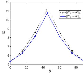
Figure 5: Effects of fiber orientation on the non-dimensional fundamental frequency for SSSS laminated UD-CNTRC plates ( $V_{CNT}^* = 0.11$ ).
