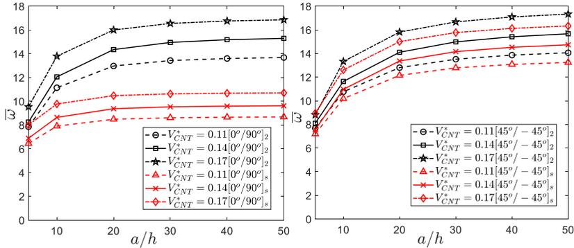
Figure 3: The change of the non-dimensional fundamental frequency of cross-ply and angle-ply laminated UD-CNTRC plates against  $a/h$  ratio with different CNT volume fractions
