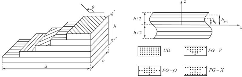
Figure 1: Geometry and configuration of laminated FG-CNTRC plate with different types of CNT distributions through layer's thickness.
