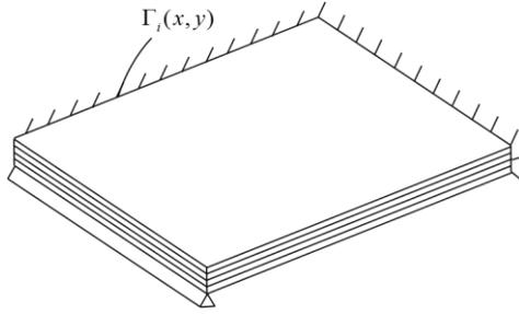
Figure 2: A rectangular laminated FG-CNTRC plate
