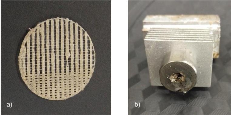
Figure 11: Results of 3D printing the PLA-OPEFBF filaments with different fibre content. a) Successfully 3D printed code 10 filament b) Clogged nozzle during 3D printing of code 30 filament.
