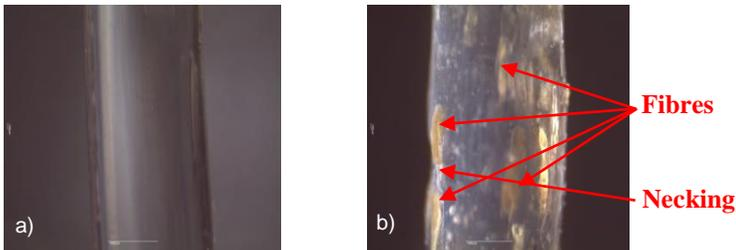
Figure 4: Microscopic image of the successfully extruded filaments (4x) a) PLA filament and b) Sample code 10 filament.
