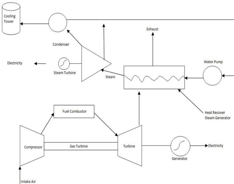
Figure 1: Working principle of single pressure CCPP.
