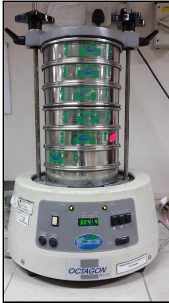
Figure 2: Mechanical sieve shaker with different mesh sizes
