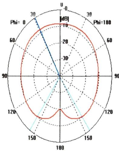
Figure 8. 2D radiation pattern of CSFA
