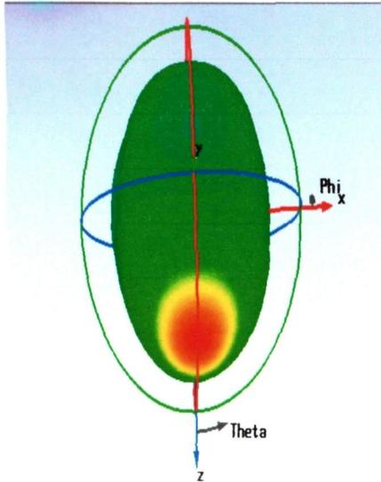
Figure 7. 3D radiation pattern of CSFA
