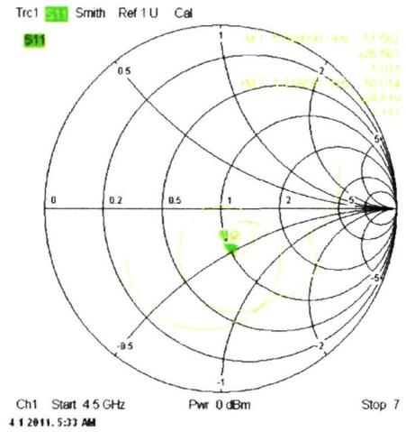
Figure 9. Measured line impedance of CSFA
