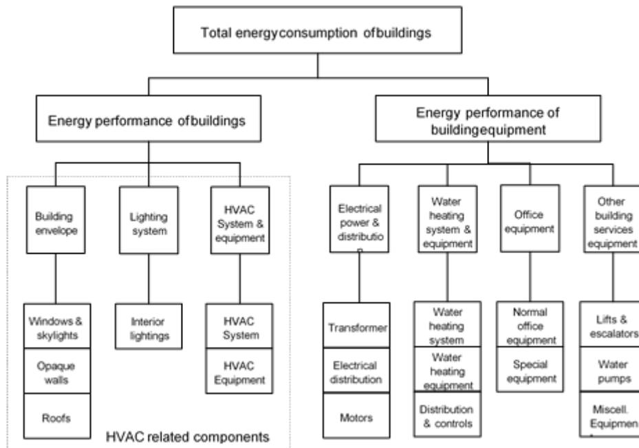
Figure 4.1 Major Components of Building Energy Consumption
