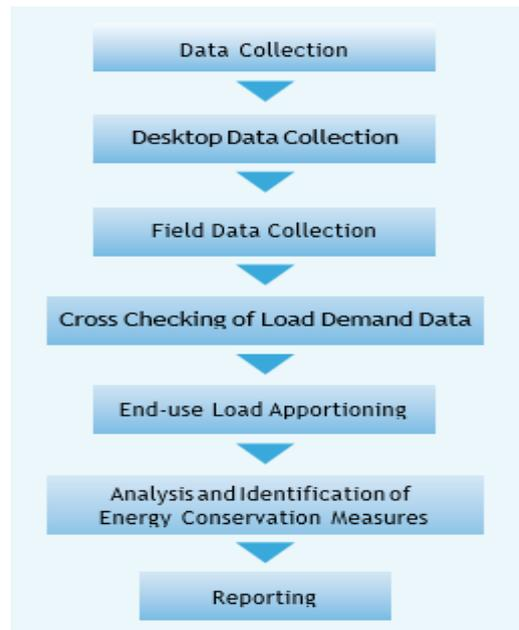
Figure 6.2 Detailed Energy Audit Process Flow
