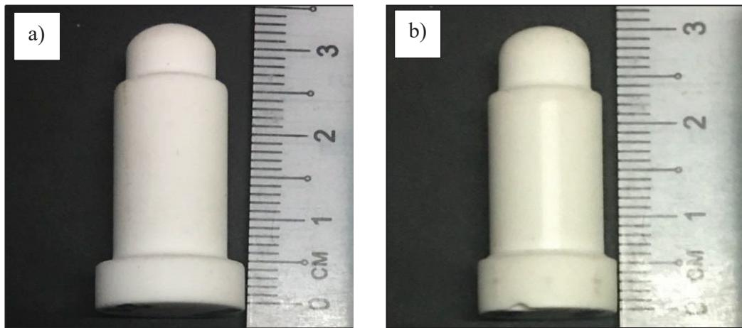
**Figure 5: Image of Model M8 Guide Pin a) Before Polishing b) After Polishing
