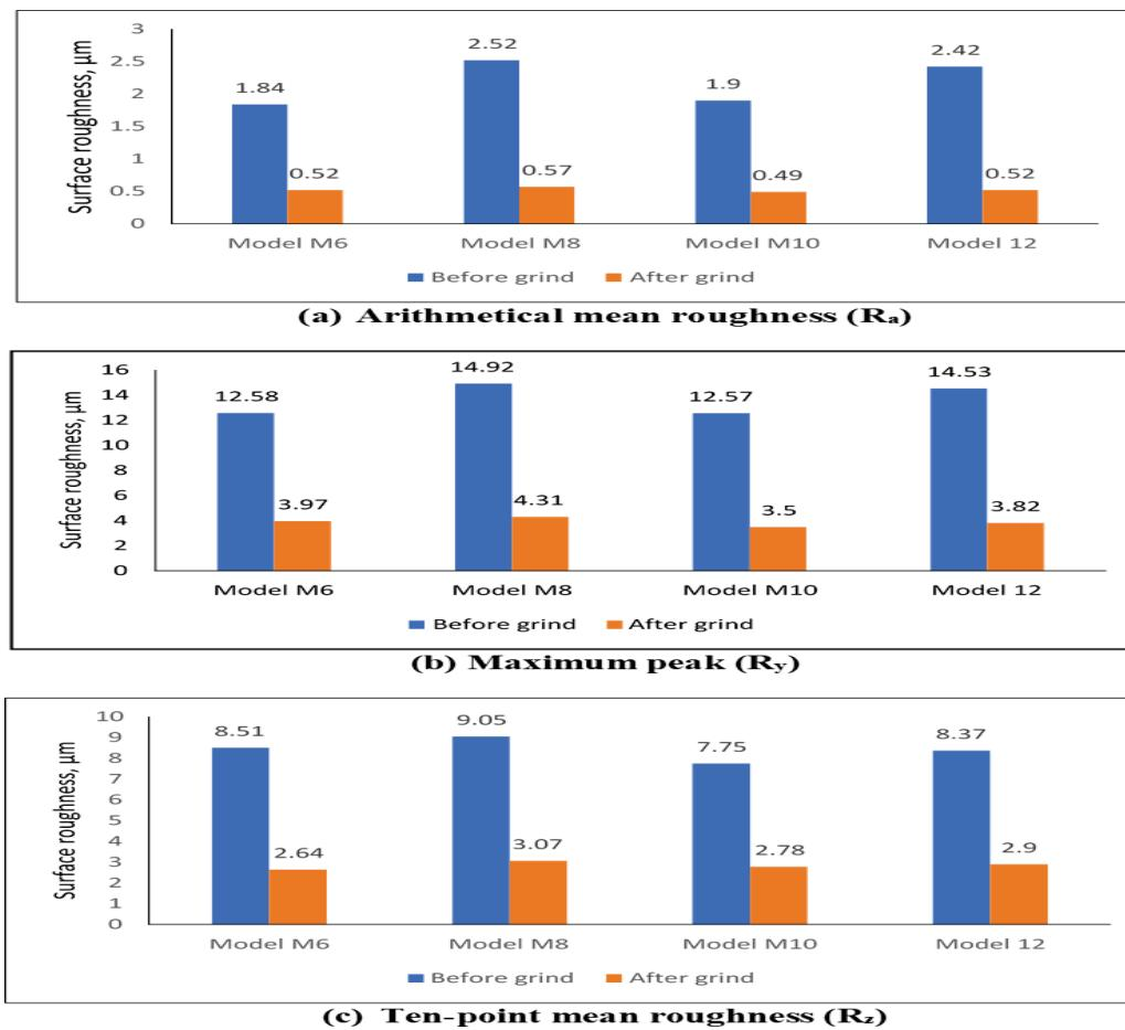
Figure 4: Surface Roughness Parameters (a)  $R_a$  (b)  $R_y$  (c)  $R_z$
