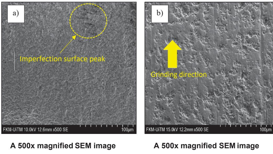
**Figure 6: SEM Image a) Before Grinding b) After Grinding**
