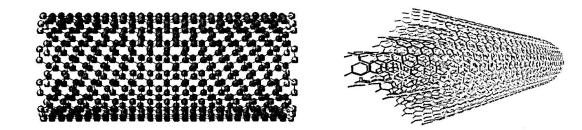
Figure 1: Single-Walled and Multi-Walled Nanotubes
