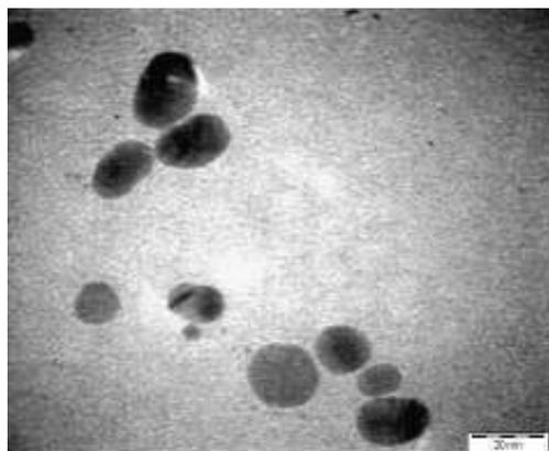
Figure 3 : TEM spectra of chemically synthesized AgNPs
