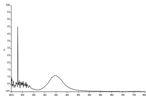
Figure 2: U.V-visible spectra of AgNPs
