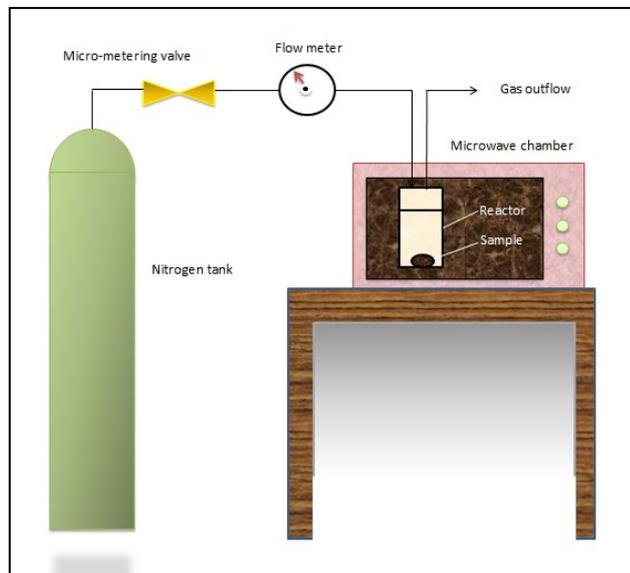
Fig. 1: Illustration on microwave pyrolysis set up for APS char activation
