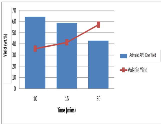
**Fig. 3:** Yield of activated charcoal against radiation time at 600 W power level
