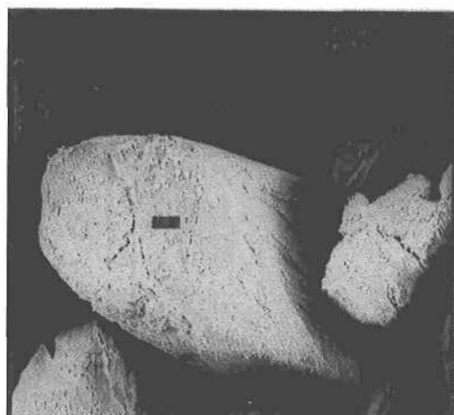
Figure 4: SEM photomicrograph of magnified spot of treated BMHA coal with PAA at 70 °C for 72 hours.
