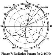
Radiation pattern is another performance of an antenna that is being studied is this research. The result of radiation patterns are being showed in figure 6 for 1.2GHz and figure 7 for 2.4GHz. From the figures, we can see that for 1.2GHz, the angular width is 96.6° and side lobe level is -19.4dB. While for 2.4GHz, the angular width is 47.8° and the side lobe level is -1.3dB.
