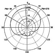
Figure 6: Radiation Pattern for 1.2GHz
