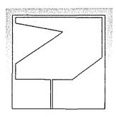
Figure 2: The extruded patch antenna
