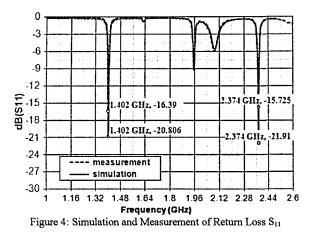
Figure 4 shows the result of return loss. From the graph, shown that the different is only with the return loss as the frequencies drop are same for simulation and measurement. For 1.402GHz, the return loss for simulation is -16.39dB while for measurement is -20.806dB. For 2.374GHz, the return loss for simulation is -21.91dB and for measurement is -15.725dB.
