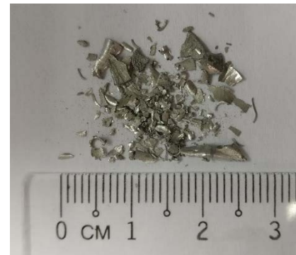
Figure 7: Blender-ed Aluminium Swarf
