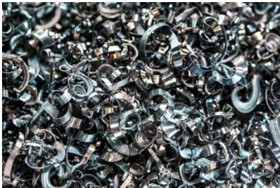
Figure 2: Aluminium metal swarf [9]
