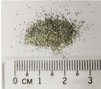
Figure 8: Sample of Pulverised Aluminium after Two Operating Cycles
