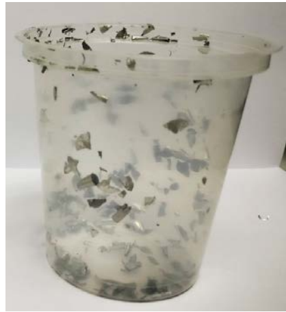
Figure 5: Soaked with lubricant aluminium swarf; sticks to container walls
