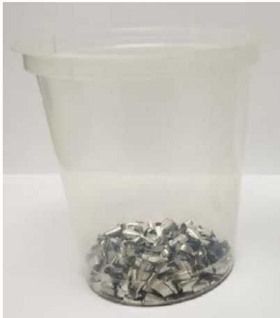
Figure 4: Cleaned Aluminium Swarf; free of lubricants (dry)
