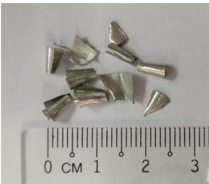
Figure 6: Cleaned Aluminium Swarf
