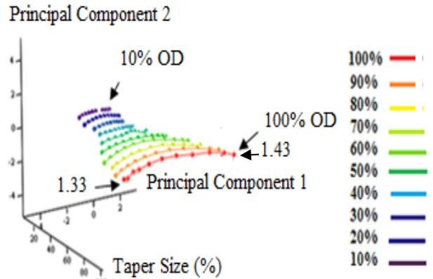
Fig. 7: 3-D score plot of a PCA model of transverse scattering pattern for taper size 10% to 100%
