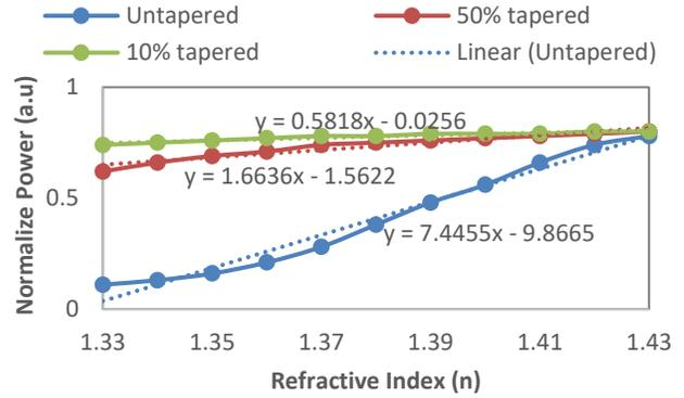
Fig. 6: Normalize power at (1.0μm) of 10%, 50% tapered, and untapered PCF
