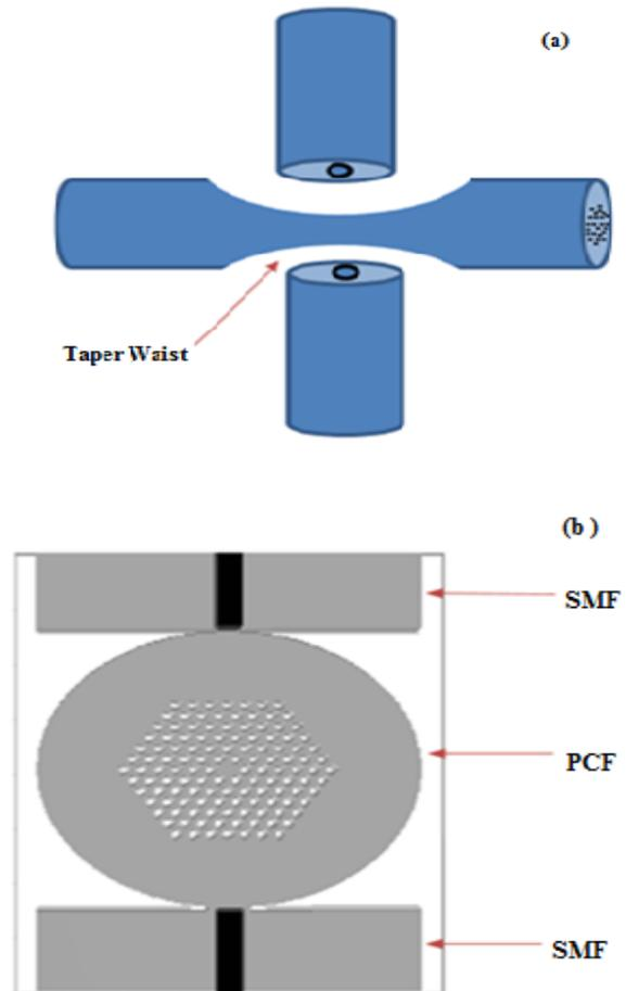
Fig. 3: (a) The tapered PCF is sandwiched between two SMF in 3D structure, (b) The design of tapered PCF is sandwiched between two SMF in 2D structure in simulation software
