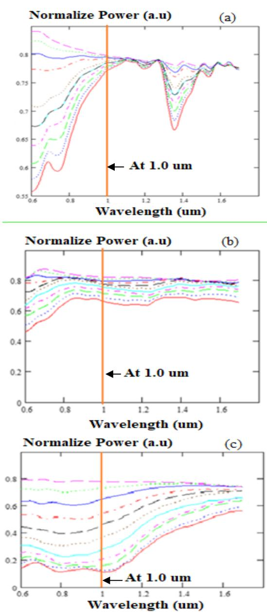
Fig. 5: (a): Scattering pattern of 10% tapered PCF, (b) scattering pattern of 50% tapered PCF, and (c) scattering pattern of untapped PCF
