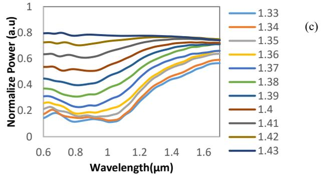
Fig. 4: (a) The transmission spectrum vs refractive index change in PCF with respect to 0.1 taper ratio, (b) The transmission spectrum vs refractive index change in PCF with respect to 0.5 taper ratio, (c) The transmission spectrum vs refractive index change in PCF with respect to untaper
